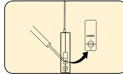
**NOTE:** When using dual wireless, each microphone must be set to a different channel!
