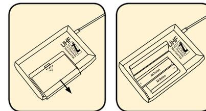
**NOTE:** Transmitter power must be OFF when changing batteries!
